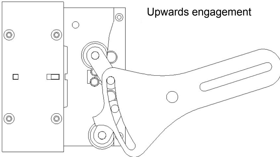
**Remark:** A circular mark in the place where the guide rails inside the safety gear are situated, will indicate the upper part of it. It is very important to make sure that the safety gears are always situated in the correct position, with the circular mark in the upper part.
