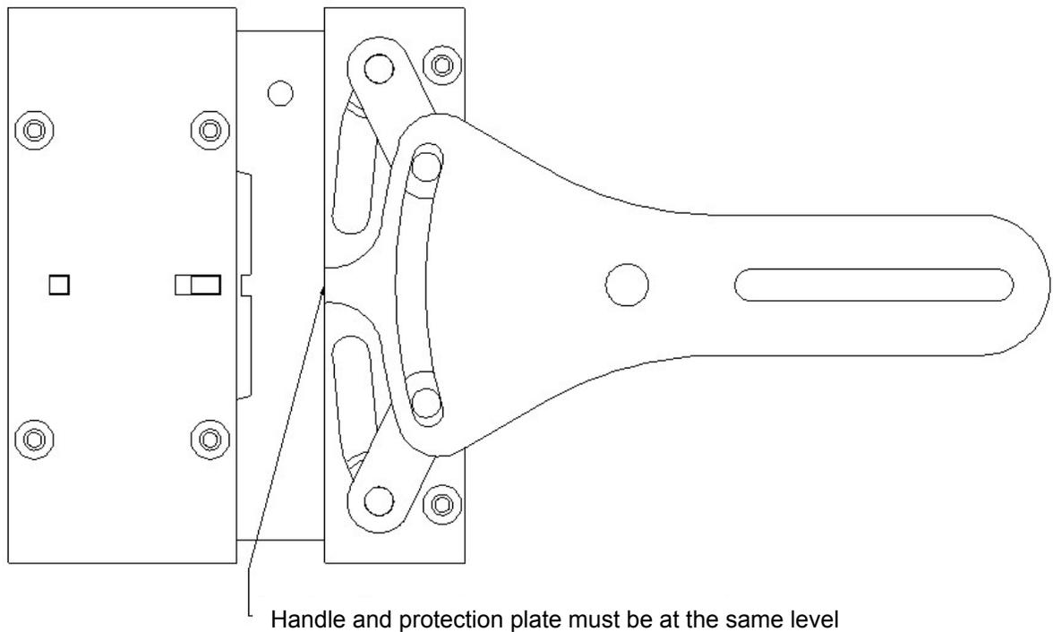
Once the safety gear is well placed and its rollers are attached to the driving bars, it should be checked that both rollers act synchronized in accordance to the driving bar commands. The sling maker is responsible for the proper location of the safety gear on the sling, as well as the adjustment checking and synchronized working of the driving bar. The
