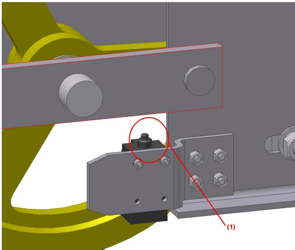
In the event of the tension loosening or even the rope breaking, the current would be cut thanks to the contact located underneath the weight-bearing bar. Due to the weight of the masses, the contact is protected from knocks by the part to which it is attached and, therefore, the sensor cannot be damaged.
