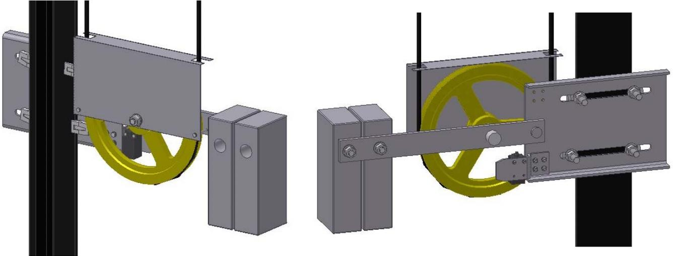
The rope must have enough tension (500 N on each side). In the event of tension loosening or rope breakage, a rope slackening contact (1) connected to the installation security series line will cut off the current.
