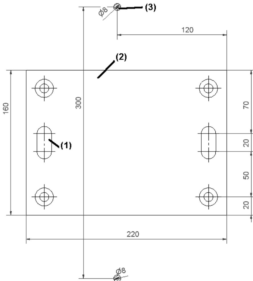
The above figure represents the bottom view of the governor base plate (2). The governor is anchored to the floor using the threaded holes (1) in the plate. The rope (3) and its position with regard to the base plate can also be seen in the drawing.
