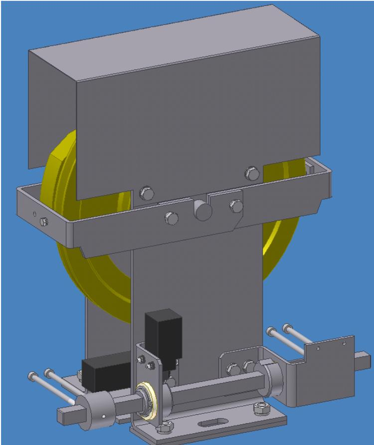
It will be provided a stops which make contact with the levers. This levers will act the security contact switch.
