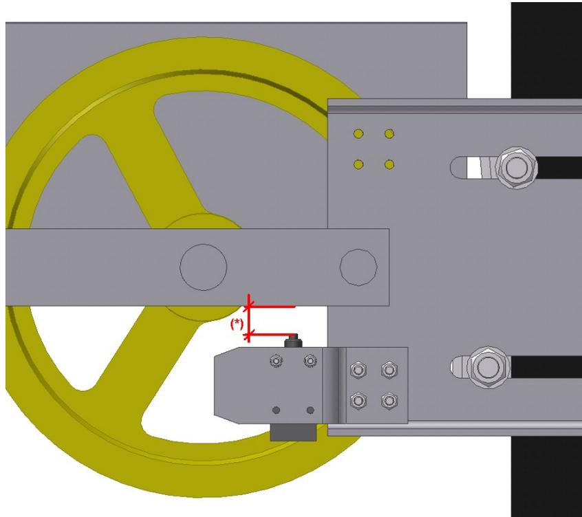
As indicated, should the tightness be less than acceptable or should the rope break, the bar supporting the weight and the pulley would make contact with the sensor.
