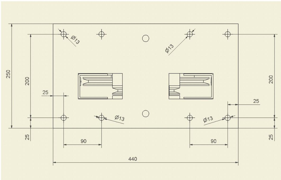
Above, it's shown the plate in order to secure the overspeed governor to the floor.
