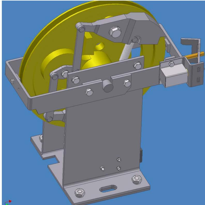
Also there is an option of acting the system without the solenoid. It is able to act manually the mechanic system, as it's shown in the figure by means of a lever.
