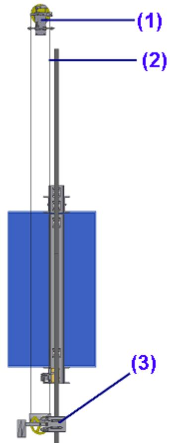
As indicated above, the governor is secured to the floor in the machine room.
