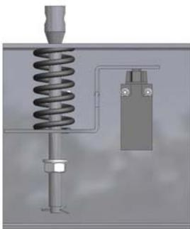
The spring is not compressed and the tensioner is supplied without any tension.
