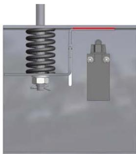
In order to know if it is being pre-tensioned in excess, we should pay close attention to the drive plate. When it touches the support, pre-tension should be reduced, as if we continue pre-tensioning, the rope will be over-tensioned without reason.
