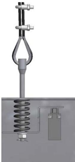
Maintaining the pre-tensioning on the rope, fit the rope ties to secure it.
