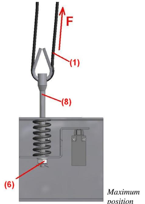
The force needed to pre-tension the rope will depend on how many metres of cable there are in the installation.
