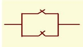
The aim of the two contacts is to detect rope breakage or detensing, as, in such a case, both springs will drive the contacts. In the case of wedging, one of the springs will loosen and the other will tighten. As a result, therefore, only one of the two contacts will open without modifying the series line.
