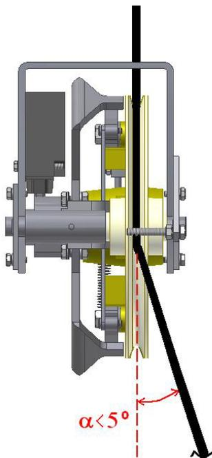
Apart from this, the rope slope is also to be taken into account, that is to say, the highest angle that the rope can form with the guide sheave.
