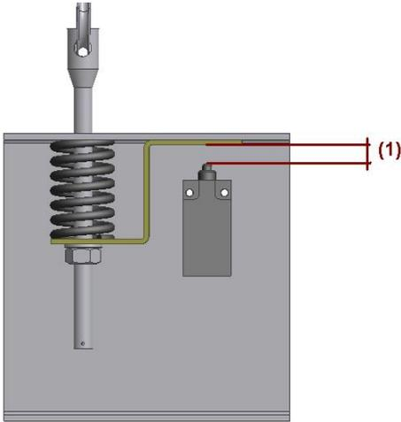
If the rope becomes loose or breaks, on recovering its natural length, the springs will allow for the plates to drive the contacts. This ensures machine stoppage.
