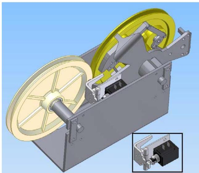
be used to release the parking system and, at the same time, unlock the governor.
