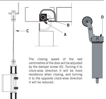
The correct adjustment is possible when the door is totally closed, softly and without banging.
