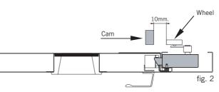
The correct distance between the wheel and the cam is 10mm. as shown in figure 2.
