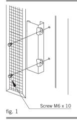
For assembling the open-door handle and pushing plate, we shuold proceed as shown in figure 1 and 2.
