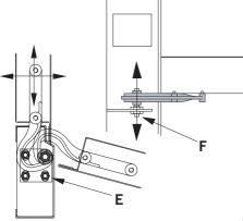
The hinges allows us to adjust the situation of the door in all directions, lateral, anterior and posterior by the slots of the subjection sheet (E). The height adjustmentis made by the axle (F) with a 6mm. "allen" key.
