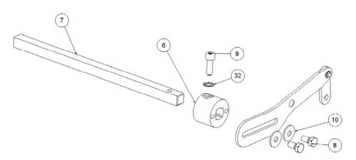
(8) and two washers DIN 9021 M8 (10), making sure that the countersink of the handle is on its inner face, – Fig. 2 –.
