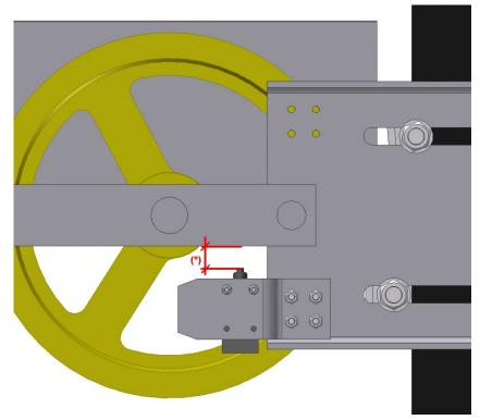
As indicated, should the tightness be less than acceptable or should the rope break, the bar supporting the weight and the pulley would make contact with the sensor.
