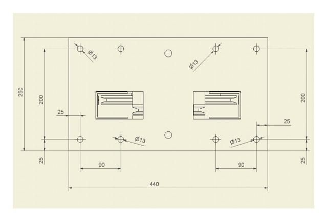
Above, it's shown the plate in order to secure the overspeed governor to the floor.
