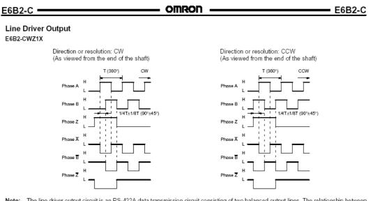
Note: The line driver output circuit is an RS-422A data transmission circuit consisting of two balanced output lines. The relationship between the two output lines is on an equal status. This means that if the level of the signal on a line is H, the level of the signal on the other line is L. The noise-resistive line driver output circuit assures high-speed data transmission.
