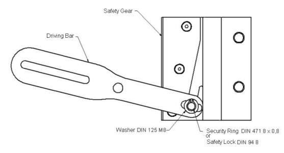
In order to the IN-4000 is replaced perfectly by the IN-6000, The instantaneous knob has to be placed a bit inclined, as it's shown in the next figure.
