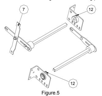
It is recommendable to fix definetively the screw after having placed the driving bar at the sling in order to improve its adjustment.
