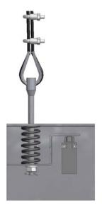
Maintaining the pre-tensioning on the rope, fit the rope ties to secure it.
