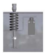
The spring is not compressed and the tensioner is supplied without any tension.
