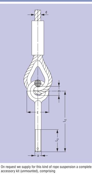
1 pressure spring, 2 spring collars, 2 nuts, 1 split pin
